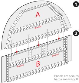
Assemble Pop-Out panels in alphabetical order. Corresponding panel edges are joined with heavier grade 2½"framework.
